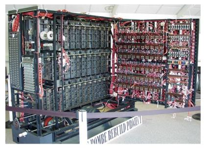
codes. This was patterned from a device called "bomba" designed in Poland by cryptologist Marian Rejewski. He had broken German Enigma messages using this device. The British bombe, like the Polish bomba, was designed to discover the daily settings of the Enigma machines in the German armed forces:
